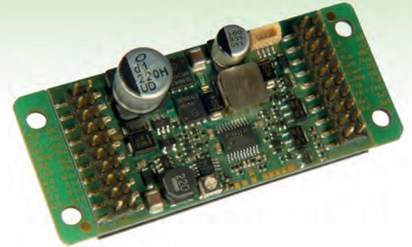
DCC + RailCom, DC-analog, MM, AC-Analog
