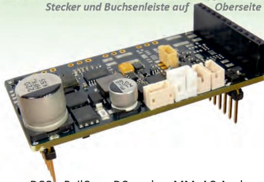
DCC + RailCom, DC-analog, MM, AC-Analog
